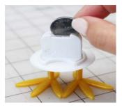
Step 3: Use a wire cutter to trim about a  $\frac{1}{2}$  inch off of each LED (10 mm big) Lead, making sure to keep the length differences. (The longer pin is positive and the shorter one is negative.)
