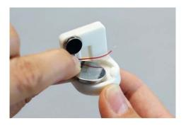
Step 4: Press the switch into place in the holder, so the pins face in towards the wires and battery. Press down on the battery when inserting the switch to ensure the battery is underneath the bottom switch pin.
