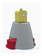
Step 4: Place a cylinder onto the Workplane. Reduce it such that its height is 21.07 and diameter is 11.40. Insert the rotatory shaft of spin cutout into the cylinder and create a hole in the cylinder.
