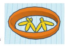
Step 2: Place the coin battery (3 Volts) in the holder with the positive side of the battery facing the same as the '+' sign on the holder.
