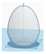
Step 4: Highlight the inner egg top only by selecting both, holding down SHIFT, and then clicking on the outer egg, which will deselect it, leaving the inner egg top still selected. Make the inner egg a hole. Step 5: Place the cylinder shape onto the workplane. Resize it such that it is 36.5 X 36.5 X 4mm.
