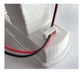
Step 4: Insert the battery box into the holder from the bottom, threading the battery wire through the hole on the side of the holder.
